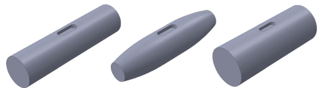
Fig. 1 Nominal (left), attacked barrel (center), and attacked diameter (right) machined cylinder
